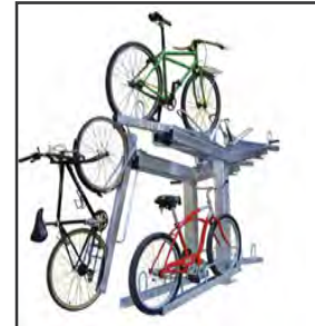
Figure 9: Two-tiered Parking Each bike should have a space 2' wide and 6' long. Each tier needs a vertical clearance of 48" (a single-tiered rack needs 96" of clearance).
