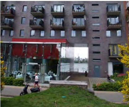
Good example of a break in the street wall to provide pedestrian access to an open space.
