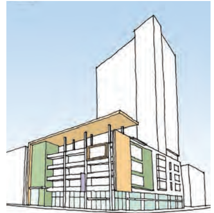
Layering with two adjacent planes that extend from the primary façade forming a modern composition.
